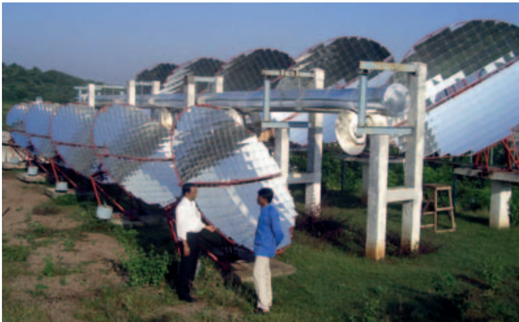
Photo 7.7 Scheffler dishes associated in pairs in a cooking system at Hyderabad (India)
