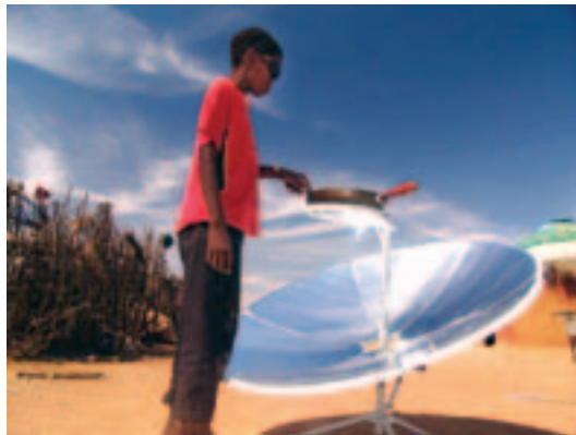
Photo 7.3 Concentrating solar cooker
